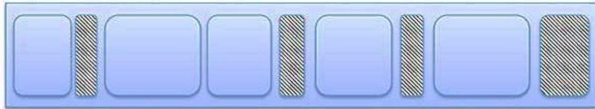
Fragmented memory before compaction
